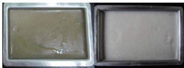
Figure 2. Experimental photos of the immobilized cells prepared for 5 min (a) and 30 min (b) UV irradiation. [Color figure can be viewed in the online issue, which is available at wileyonlinelibrary.com .]
